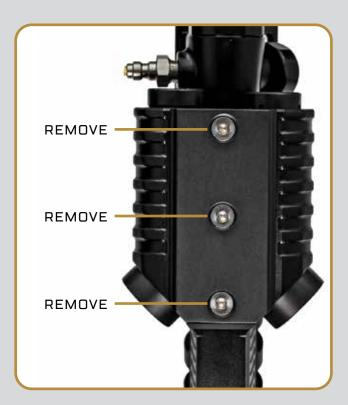
Remove the **3 bolts** that secure the ARCA rail attachment. The standard short rail & the longer match rail have the same mount location & hardware.
