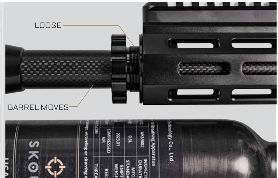
BARREL LOCK LOOSE
