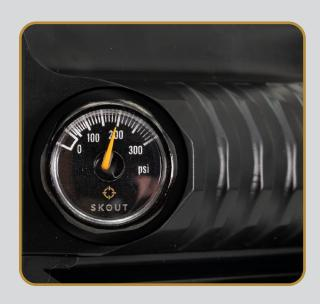
This is your Low Pressure Regulator (LPR) reading. This pressure represents the force used to open and close the valve.
